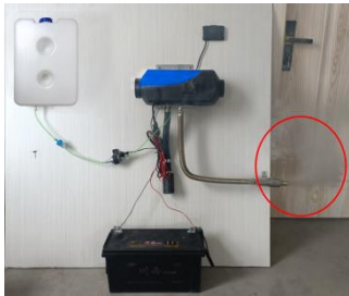
Excessive pump oil produces white smoke
